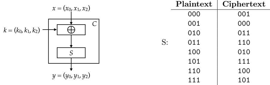
In particular,  $C$  maps a 3-bit input block  $x = (x_0, x_1, x_2)$  to a 3-bit output block  $y = (y_0, y_1, y_2)$  using a 3-bit key  $k = (k_0, k_1, k_2)$  and a function  $S$  as follows:
